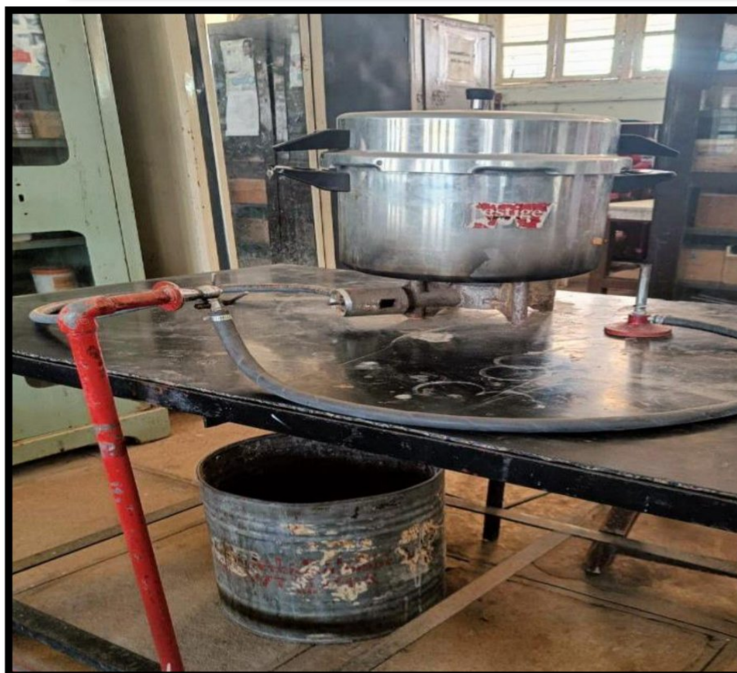
Pressure Cooker For Decontamination of Pathogen & sterilization of Culture Media
