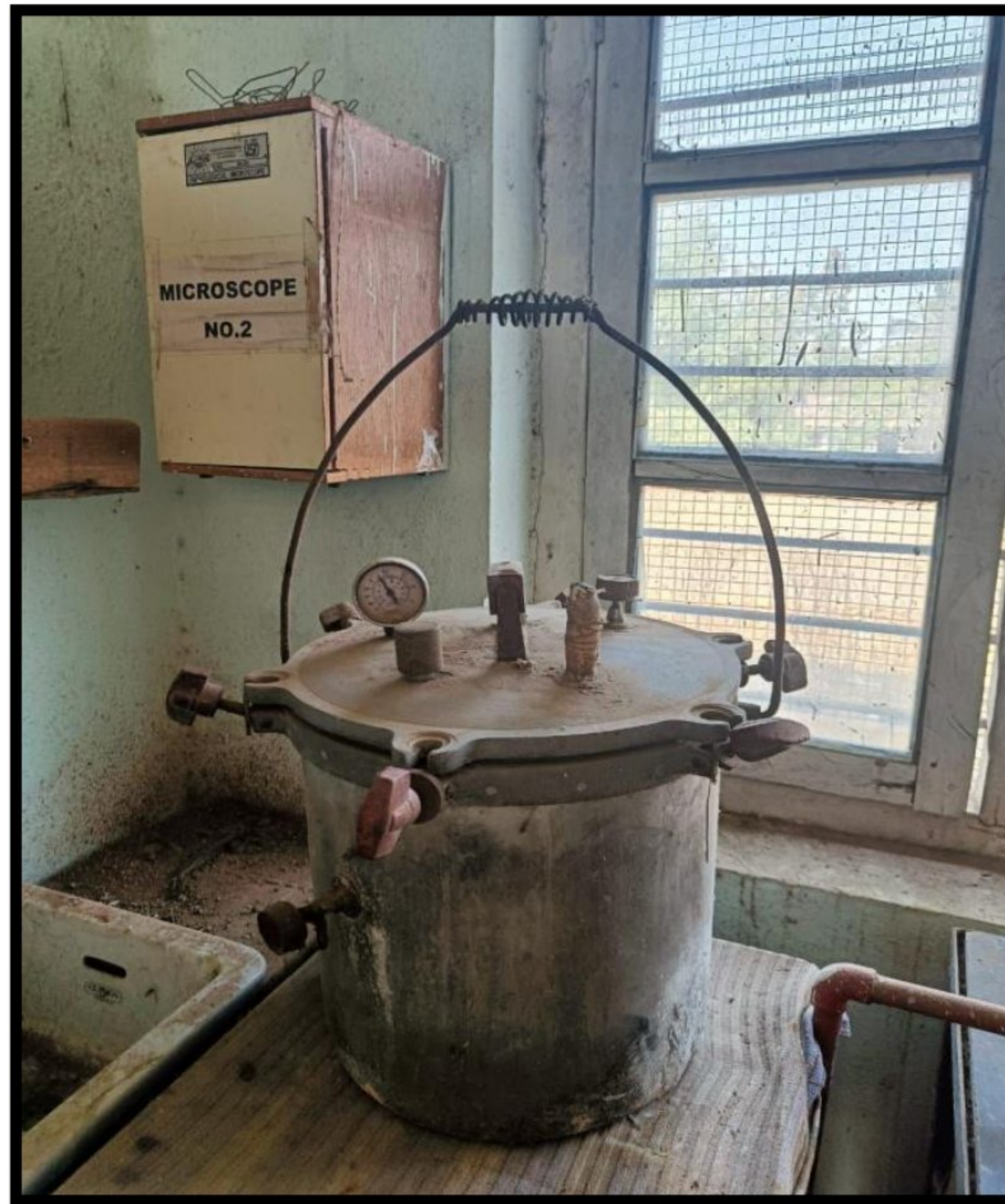
Autoclave For Decontamination of Pathogen & of Culture Media
